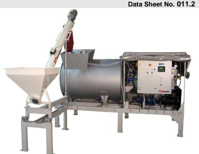
Use: The MS 1000S is designed for operation in automatic mode while it can simultaneously control three conveyors for accurate re-dosing of two dry components as a minimum.
