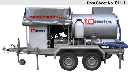
The manufacturing process has two phases. First, the raw materials are automatically fed into the mixer and are thoroughly, automatically mixed; wherein the dosage of water, chemical admixture and cement takes place simultaneously, followed by sand (if required) and the preformed foam. Polystyrene beads and Fibre (if required) are dosed manually.
